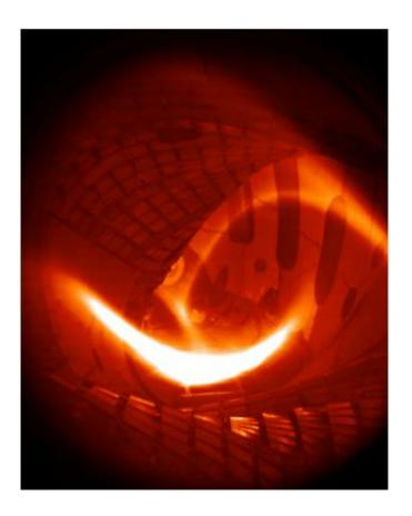
Helically twisted plasma glows during the first hydrogen operation in W7-X on Feb. 3, 2016. Credit: Max-Planck Institute for Plasma Physics
