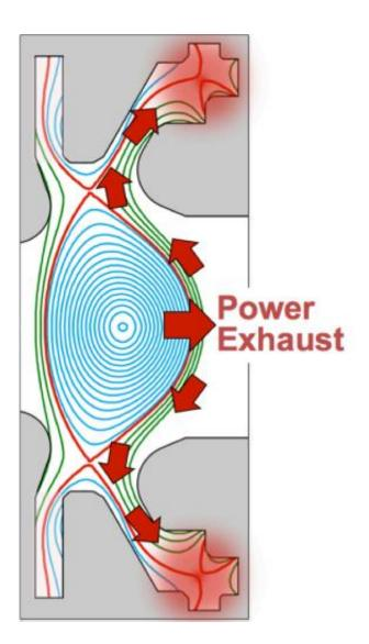
Cross-section of a tokamak plasma, with cylindrical symmetry axis at left side, showing a potential solution to the fusion power exhaust challenge: (1) topbottom symmetric core plasma, defined by magnetic x-points and (2) specially designed, long-leg exhaust channels to dissipate the power via radiation,
