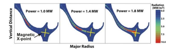
Simulation of power exhaust and radiation in a long-leg plasma exhaust channel that contains a secondary magnetic x-point. Plasma heat exhaust is fully accommodated by a passively-stable radiating layer, keeping the hot plasma from coming into contact with material walls. As exhaust power is increased, the location of radiating layer moves down the leg. The embedded magnetic x-point acts as a backstop to handle the most intense power levels. Credit: MIT
