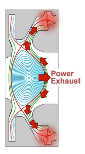
Cross-section of a tokamak plasma, with cylindrical symmetry axis at left side, showing a potential solution to the fusion power exhaust challenge: (1) top-bottom symmetric core plasma, defined by magnetic x-points and (2) specially designed, long-leg exhaust channels to dissipate the power via radiation,
