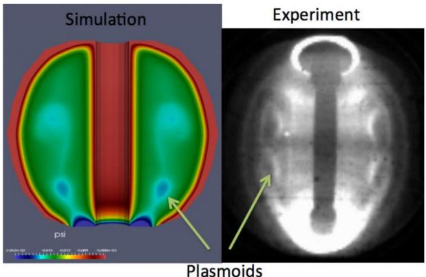
Left: Plasmoid formation in simulation of NSTX plasma during startup without solenoid. Right: Fast-camera image of NSTX plasma shows two discrete plasmoid-like structures. Credit: NSTX
