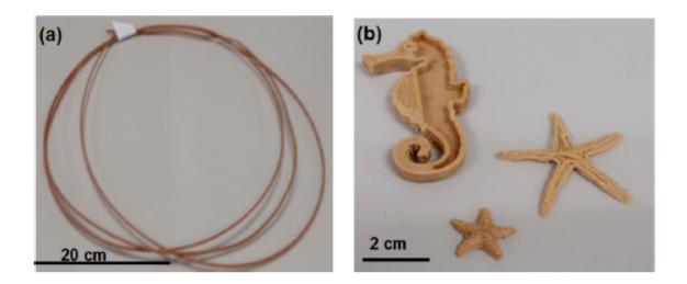
New directions in 3D technology- filaments produced by hot-melt extrusion. Credit: University of Melbourne
