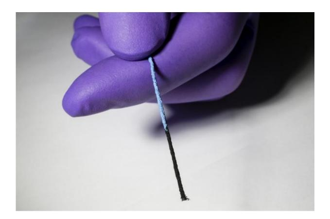
A hydro-responsive thread can be used with sensors to monitor body functions. Credit: Alonso Nichols, Tufts University, CC BY-ND
