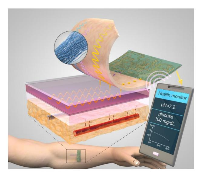
Smart threads can monitor wounds using a suite of physical and chemical sensors made using threads and passing information to a skin-surface transmitter. Credit: Nano Lab, Tufts University, CC BY-ND
