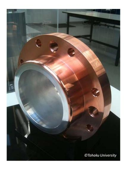
Thick deposit of copper (between 50 to 60 mm) obtained by "Cold spray." The deposited copper is machinable: holes for screws, flanges, etc. Credit: Tohoku University
