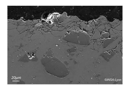
Spread of corrosion in a coating obtained by "Cold spray". Credit: INSA-Lyon.
