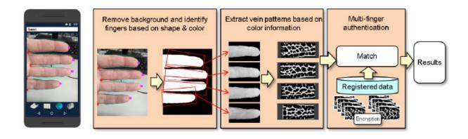
Finger vein authentication technology using smartphone camera. Credit: Hitachi
