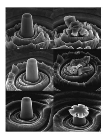
Scanning electron microscope images show pristine (left) and compressed (right) micropillars of (top) chromium nitride, (middle) chromium aluminum nitride, and (bottom) chromium aluminum nitride / silicon nitride nanocomposite. Credit: AIP Publishing
