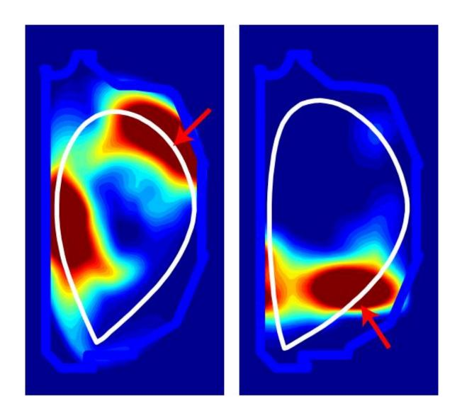
Comparison of experimentally measuredradiated power emission patterns inside the DIII-D tokamak with upper gas injection (left) and lower gas injection (right). Arrowsindicates gas valve locations, the whiteborder represents the plasma boundary, and the light blue border shows the vacuumvessel. Red coloring indicates the strongestemission, blue weakest. Credit: General Atomics
