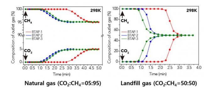
This data presents the breakthrough measurements for  $CO_2$ -containing binary gas-mixture streams with different feed-gas compositions to investigate the  $CO_2$  capture capacity of ultramicroporous benzothiazole polymers (BTAPs) for large-scale applications under simulated conditions of natural and landfill gases. Credit: KAIST
