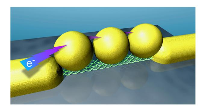
The DNA itself has no part in the electrical function, but acts as a scaffold for forming a linear, pearl-necklace-like nanostructure consisting of three gold nanoparticles. Credit: the University of Jyväskylä
