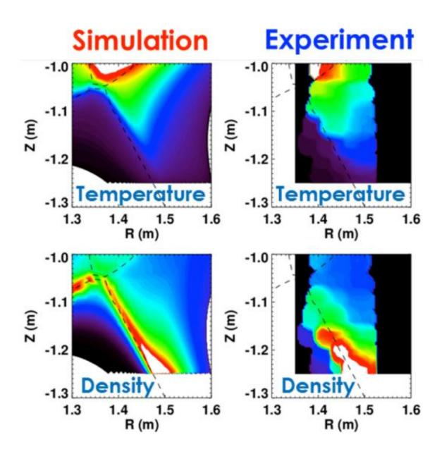
Simulationsreproduce the plasma temperature (top) and density (bottom) in the divertor region. Credit: ORNL
