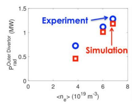
The high radiation levels found in tokamak experiments are also found in simulations Credit: ORNL
