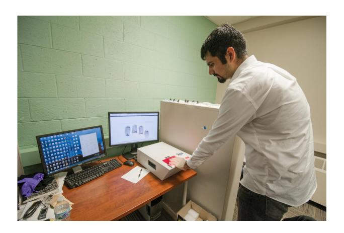
MSU doctoral student Sunpreet Arora demonstrates how a 3-D printed model hand is used to test a fingerprint scanner for accuracy. Credit: G.L. Kohuth
