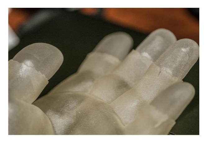
MSU researchers demonstrate how a 3-D printed model hand is used to test a fingerprint scanner for accuracy. Credit: G.L. Kohuth
