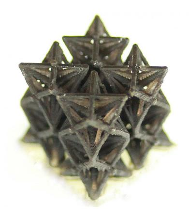
While most solid materials expand with heat, this 3-D-printed structure, designed by MIT engineers, is designed to shrink, based on the stretching and pulling of its internal beams and trusses. Credit: Qiming Wang
