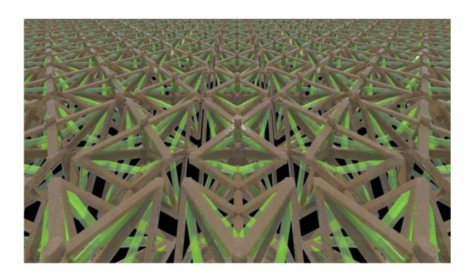
LLNL researchers were part of a team that demonstrated a bi-material microlattice structure, 3D printed from polymer and a polymer/copper composite material, that can flex inward, causing the structure to contract when exposed to heat over a range of tens to hundreds of degrees. Credit: Lawrence Livermore National Laboratory
