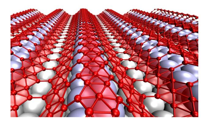
When grown on silver, the two-dimensional form of boron, which is called borophene, takes on corrugations. The metallic material may be suitable for use in stretchable, bendable electronics. Credit: Zhuhua Zhang/Rice University
