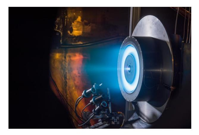
Miniaturized ion engines are a method of choice for providing thrust control for CubeSats. Credits: NASA
