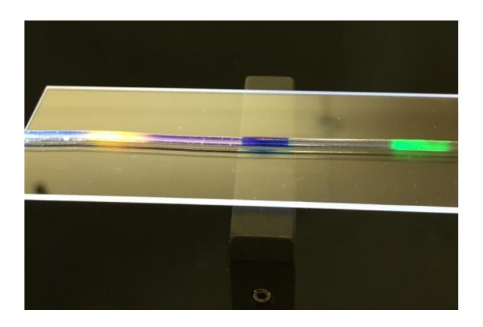
MIT researchers have developed a stretchy optical fiber in which they have injected multiple organic dyes (yellow, blue, and green regions). In addition to lighting up, the dyes act as a strain sensor, enabling researchers to quantify where and by how much a fiber has been stretched. Credit: Massachusetts Institute of Technology
