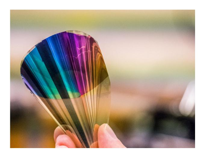
Chalmers' e-paper contains gold, silver and PET plastic. The layer that produces the colours is less than a micrometre thin. Credit: Mats Tiborn
