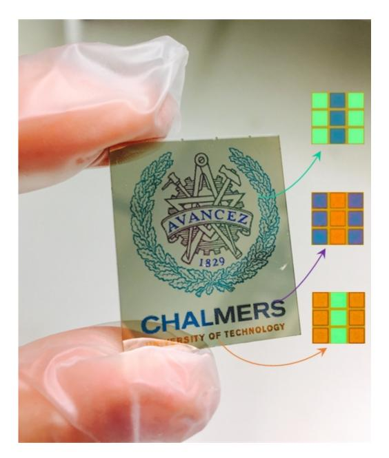
Researchers at Chalmers University of Technology have developed the basis for a new electronic 'paper'. Chalmers' logotype shows how the RGB pixels can reproduce color images. The magnification shows which pixels are activated to create the image. Credit: Kunli Xiong
