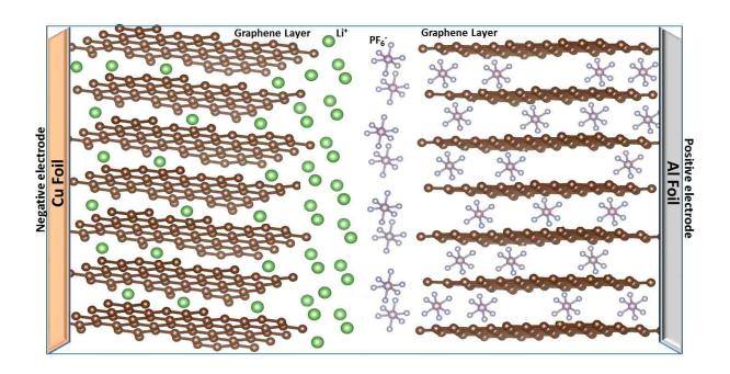
In dual-ion batteries, upon charging, anions migrate into the lattice of the positive electrode and cations move into the structure of the negative electrode. Credit: Oregon State University
