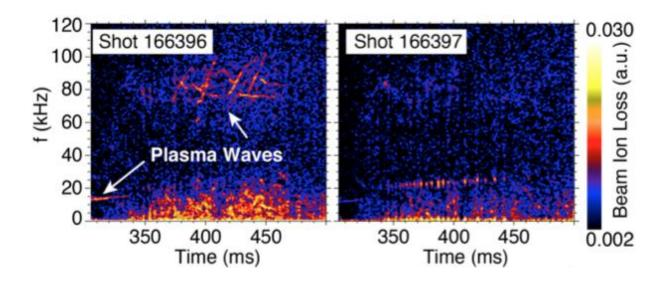
Spectrograms of measured beam ion loss. Both plasma shots feature the same total beam power, but the shot shown on the right utilizes a beam voltage program that greatly reduces the amplitude of coherent plasma waves. Credit:
