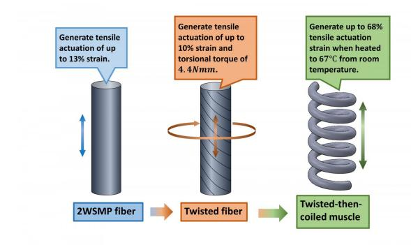
This is the fabrication procedure and actuation of coiled artificial muscle based on two-way shape memory polymer fiber. Credit: Louisiana State University
