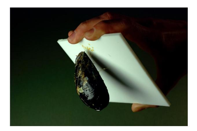
Researchers are working on a new environmentally friendly method to control tenacious shellfish that attach to the hulls of ships, increasing drag and hiking fuel consumption by as much as 50 percent. Here, a mussel is attached to a sheet of Teflon. Credit: Purdue University photo/Jonathan Wilker
