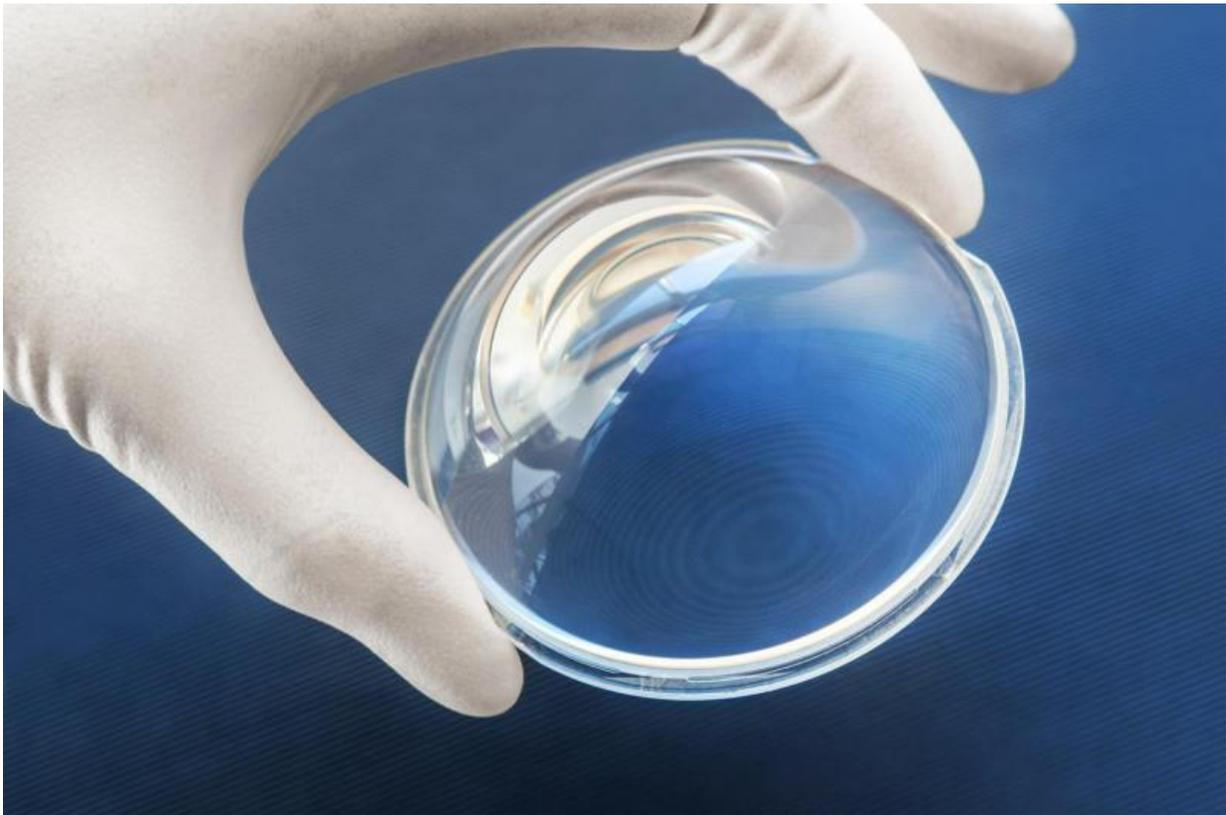
Injection-molded optical lens made from transparent plastic demonstrating the nanostructured antireflective coating. Only the coated right half shows the effect of the antireflection system. The uncoated left half reflects the light. Credit: Fraunhofer IOF
