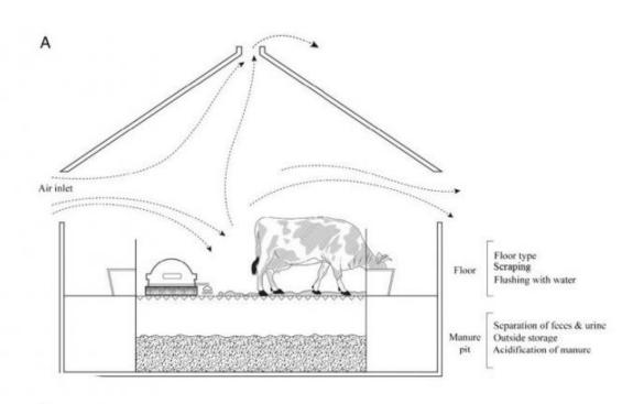
NH3 emission mitigation techniques include floor type, floor scraping and flushing with water, and acidification of manure. Credit: Mendes *et al* (2017)
