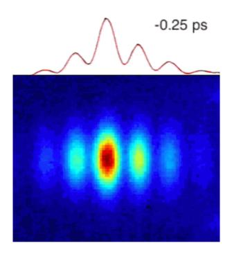
This movie shows how a laser pulse hitting a chromium crystal causes charge density waves – alternating areas of high and low electron density within the crystal – to oscillate in height, or amplitude. The signal seen here is made by X-ray laser pulses scattering off the crystal. The timescale of the oscillations is shown in picoseconds, or trillionths of a second. Credit: A. Singer/University of California, San Diego
