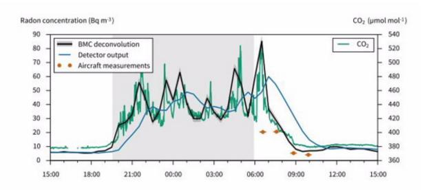
Field observations from a calm and clear night on the 5th–6th of November 2011. The wind speed was <sup>-1</sup> at 2 m a.g.l. for most of the night. Aircraft measurements were made 36–41 m .a.g.l. over 6 km flight segments. Night-time is shaded grey, as is the 16th–84th percentile range about the reconstructed time series. Credit: Australian Nuclear Science and Technology Organisation (ANSTO)
