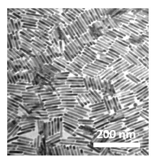
Transmission electron microscope image shows lead telluride (PbTe) nanorods developed by materials scientists at the Georgia Institute of Technology using a new strategy for crafting one-dimensional nanorods from a wide range of precursor materials. Credit: Georgia Tech
