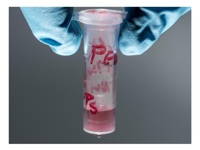
Image shows a vial containing water-soluble gold nanorods. Georgia Tech researchers have developed a new strategy for crafting one-dimensional nanorods based on cellulose using a wide range of precursor materials. Credit: Rob Felt, Georgia Tech
