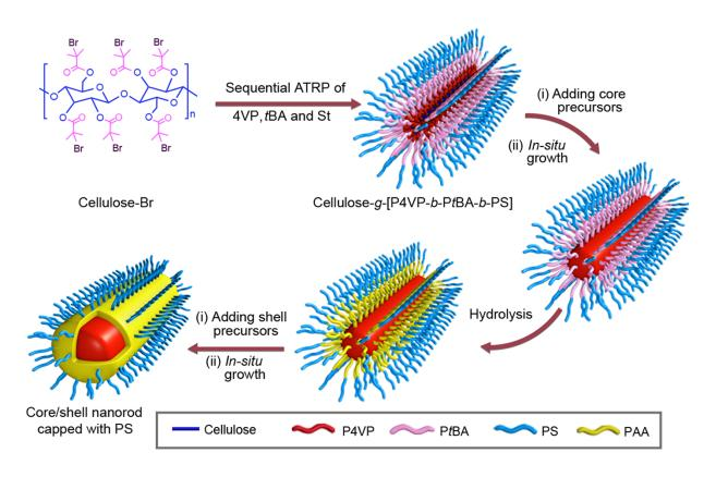
Schematic shows the steps involved in producing oil-soluble core-shell nanorods capped with polystyrene. Credit: Georgia Tech
