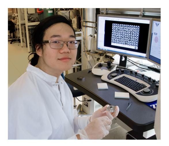
Summer Scholar Justin Cheng holds an experimental sample of nanostructured gold on silicon that has potential for use in sensors and display technologies based on its selective light absorption properties. Credit: Maria E. Aglietti/Materials Processing Center
