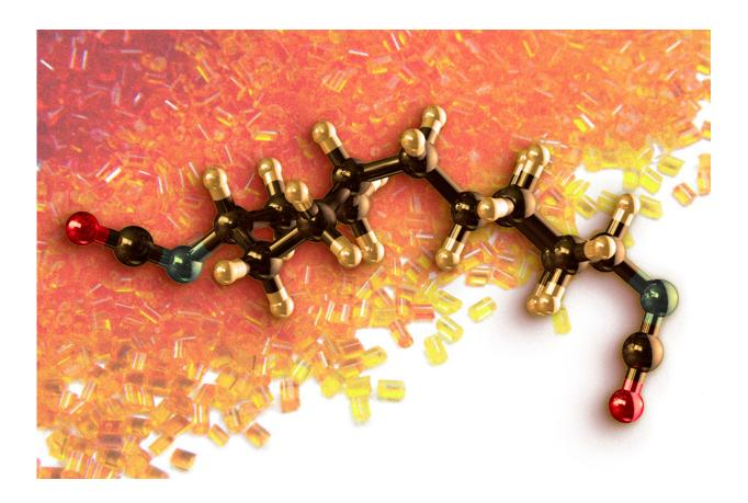
Polymers, or long chains of repeating molecules, are found in many objects that we encounter every day, including anything made of plastic or rubber. In many materials, however, a significant fraction of these chains bind to themselves, forming defects. Credit: Jose-Luis Olivares/MIT
