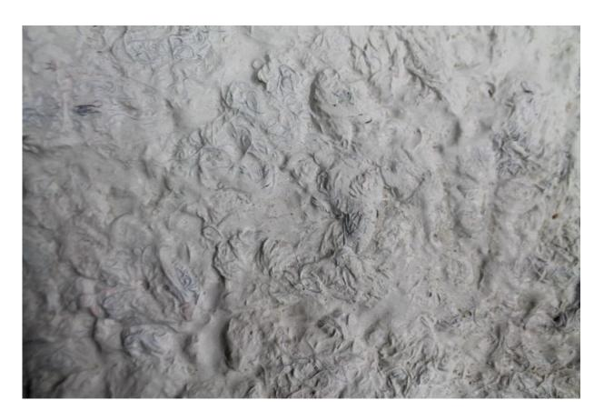
Textile fiber panel bindered with natural hydraulic lime. Credit: UPM
