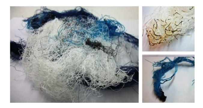
Textile waste used to build the panel. Credit: UPM
