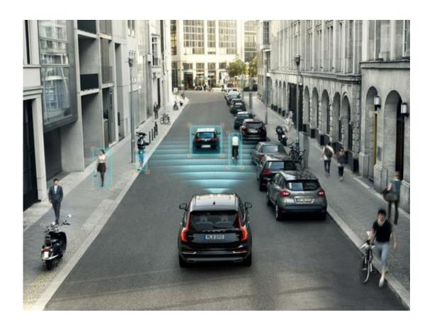
This undated photo rendering provided by Volvo Cars shows the car makers City Safety feature in one of their XC90 SUVs. City Safety features pedestrian and cyclist detection with full auto brake, day and night. (Volvo Cars via AP)
