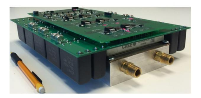
The new inverter, made using silicon carbide components. Credit: Iqbal Husain.
