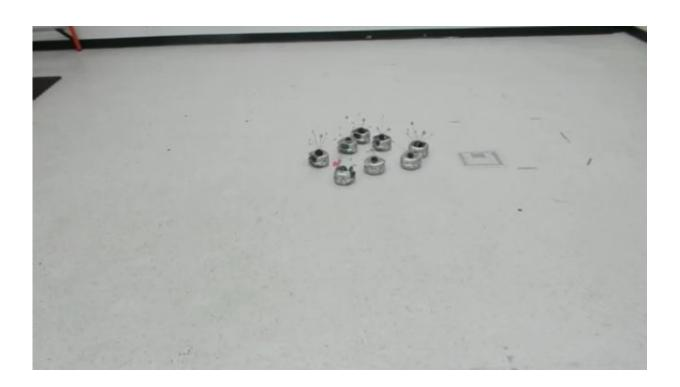
When roboticists create behaviors for teams of robots, they first build algorithms that focus on the intended task. Then they wrap safety behaviors around those primary algorithms to keep the machines from running into each other. Each robot is essentially given an invisible bubble that other robots must stay away from. As long as nothing touches the bubble, the robots move around without any issues. But that's
