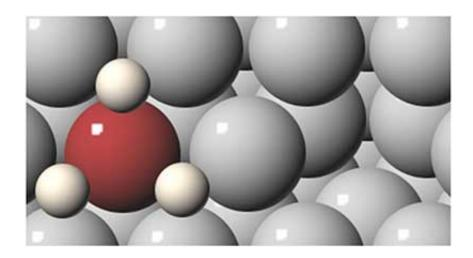
This reaction diagram models the interaction of hydrogen (red sphere) and titanium (white sphere) with aluminum (gray spheres) to form alane. A vacancy in the aluminum surface is shown on the right. Credit: U.S. Department of Energy
