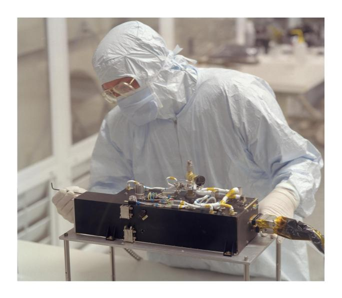
The SwRI-developed Alice ultraviolet spectrograph, shown here during final integration, collected more than 70,000 spectra during a 2-year mission orbiting comet 67P/Churyumov-Gerasimenko. The instrument performed flawlessly
