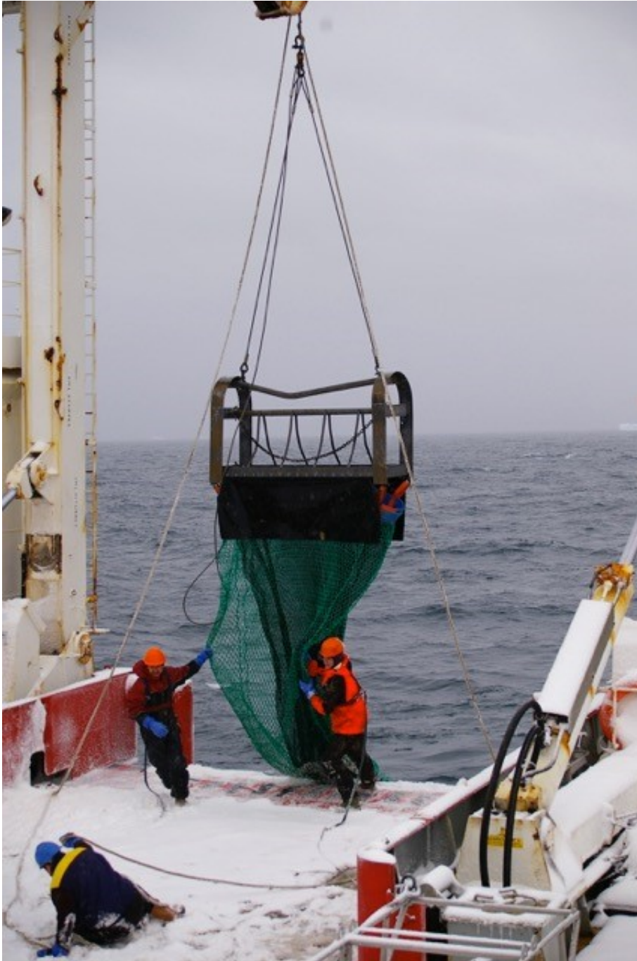
An Agassiz trawl on board the RRS James Clark Ross. Credit: British Antarctic Survey
