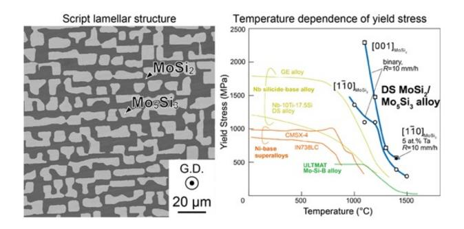
Figure (left): Electron micrographs of directionally solidified (DS) ingots of binary composites. (right): Temperature dependence of yield stress of DS MoSi2/Mo5Si3 eutectic composites and some high-temperature materials. Credit: Hirotaka Matsunoshita, Yuta Sasai, Kosuke Fujiwara, Kyosuke Kishida and Haruyuki Inui.
