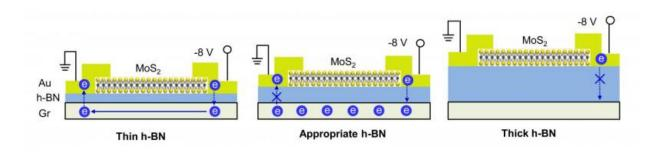
The appropriate thickness of the h-BN isolating layers allows electrons to tunnel and reach the graphene layer without leakages. H-BN layers of different thicknesses were tested and a thickness of 7.5 nanometers was found to be the most appropriate. Credit: Institute for Basic Science
