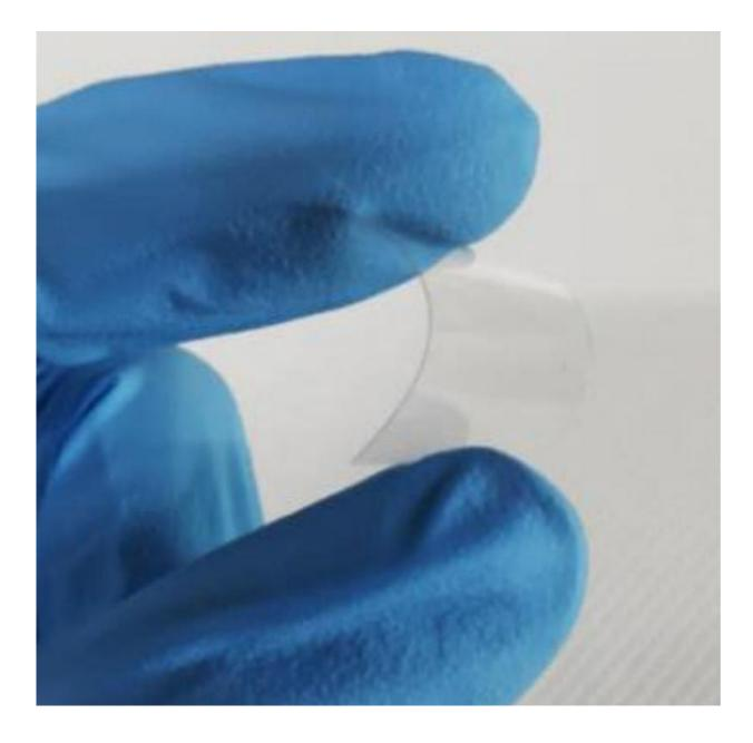
Two-terminal tunnelling random access memory (TRAM) shows good flexibility when built on flexible polyethylene terephthalate (PET). TRAM can be useful for next-generation wearable or body-attachable soft devices. Credit: Institute for Basic Science
