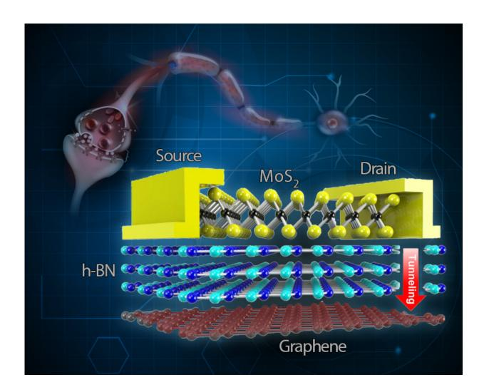
Comparison between the synapse and the two-terminal tunnelling random access memory (TRAM). In the junctions (synapses) between neurons, signals are transmitted from one neuron to the next. TRAM is made by a stack of different layers: A semiconductor molybdenum disulfide (MoS2) layer with two electrodes (drain and source), an insulating hexagonal boron nitride (h-BN) layer
