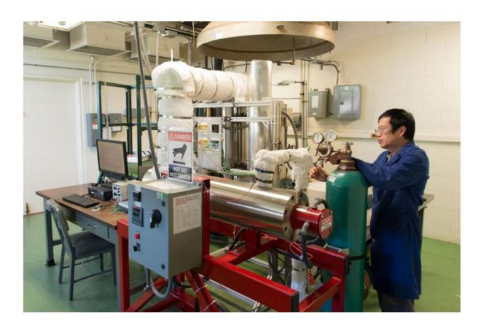
Argonne National Laboratory mechanical engineer Wenhua Yu prepares to test a prototype thermal energy storage system developed at Argonne that will charge and discharge 20 times faster than current high-efficiency latent heat thermal energy storage systems. Testing validates the amount of thermal energy that can be stored and how efficiently it can be recovered for concentrated solar power and other potential applications. Credit: Argonne National Laboratory
