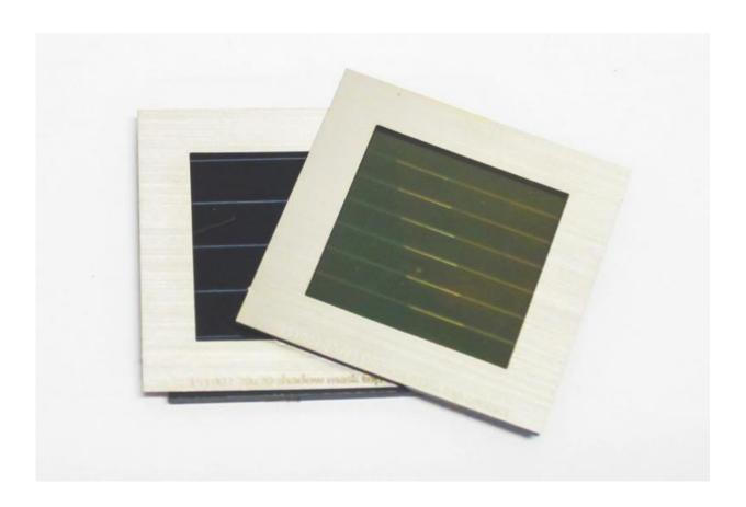
Caption: The two thin-film modules of the highly efficient stack: CIGS below, perovskite on top. Credit: IMEC
