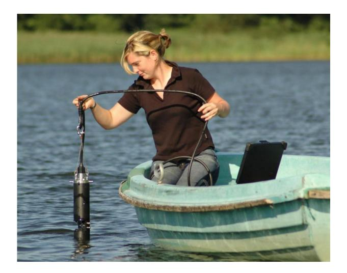
Current way of using the multi-algae sensor. In the future, it will be operated auto-matically from buoys together with other sensors. Credit: bbe Moldaenke
