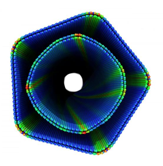
Superposition of two double-wall nanotubes with different structural conformation following the relative chiralities: monochiral (internal nanotube) and polychiral (external nanotube) Credit: SISSA/CNR IOM
