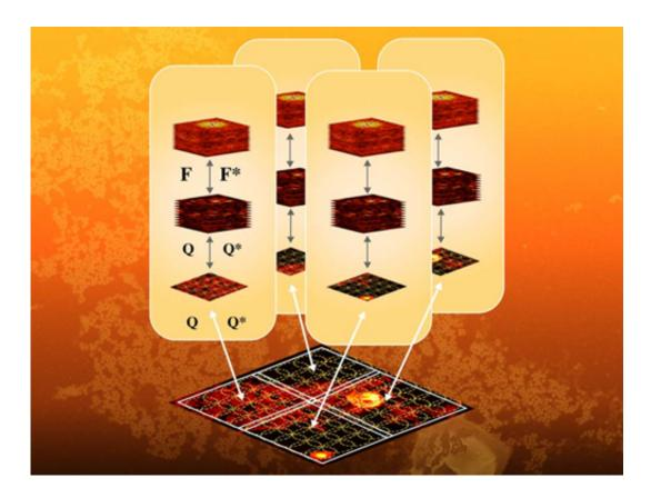
In ptychography, the x-ray beam scans through the sample, creating diffraction data (a frame) for each point. SHARP distributes the large dataset and workload onto many parallel GPU (graphics processing unit) cores to produce very high resolution images in less then a second. Credit: Lawrence Berkeley National Laboratory
