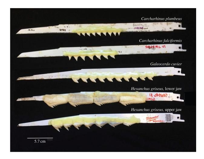
Shark teeth were attached to reciprocating saw blades using epoxy. Credit: University of Washington
