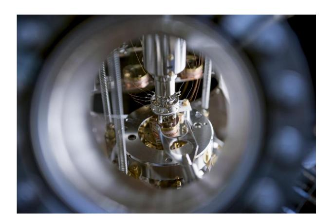
The Scanning Tunnelling Microscope used to inject electrons into a silicon surface at the University of Birmingham. Credit: Michelle Tennison
