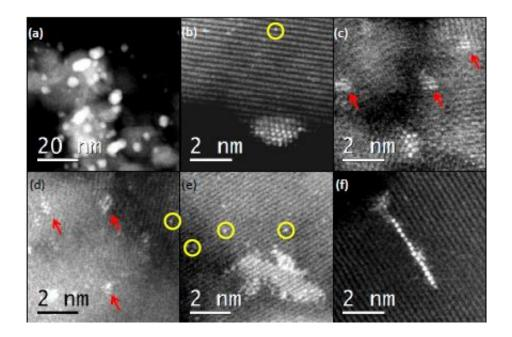
Supported gold catalysts when observed with Lehigh's aberration-corrected STEM microscope show the co-existence of several Au species that could be potentially active for CO oxidation. These include isolated atoms (yellow) and sub-nanometer clusters (red) as well as epitaxial nanoparticles, ordered monolayer rafts and linear stripes. Credit: Christopher Kiely et al
