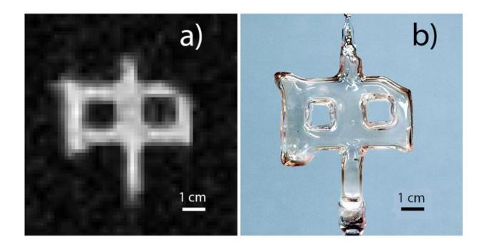
Photo A is an image of a sealed glass cell obtained by UVA physicists by combining magnetic-resonance techniques with the detection of gamma rays emitted by an isotope of xenon contained within the cell. Image B is an ordinary photograph of the glass cell. Credit: University of Virginia
