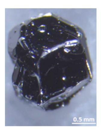
A single crystal of cadmium arsenide. Single crystals of this material, known as a "Dirac semimetal," were cut to form nanoscale slices. The slices, when exposed to a magnetic field, exhibited an odd, roundabout electron path. The material
