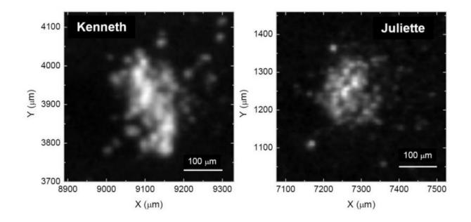
Optical image of two of the dust grains collected and analysed by COSIMA, named Kenneth and Juliette, which show the signature of carbon-based organics. They were collected in May and October 2015 respectively. Credit: ESA/Rosetta/MPS for COSIMA Team MPS/CSNSM/UNIBW/TUORLA/IWF/I AS/ESA/BUW/MPE/LPC2E/LCM/FMI/UTU/LISA/UOFC/vH&S/ Fray et al (2016)
