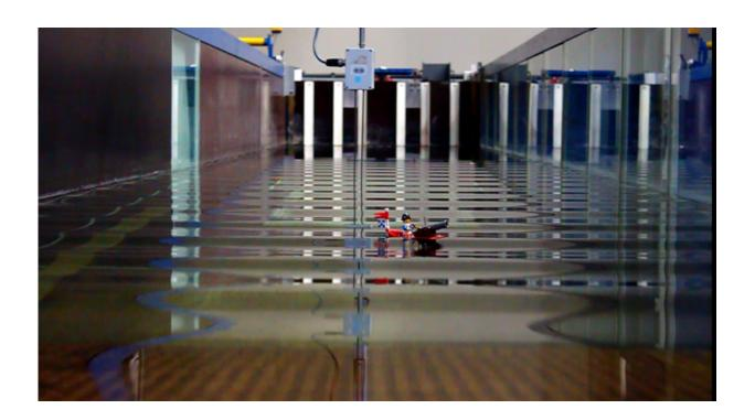
Potentially extremely dangerous realistic rogue waves can now be controlled and generated at will in laboratory environments. Credit: Hamburg University of Technology
