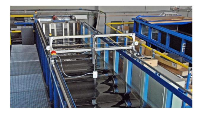
Potentially extremely dangerous realistic rogue waves can now be controlled and generated at will in laboratory environments. Credit: Hamburg University of Technology
